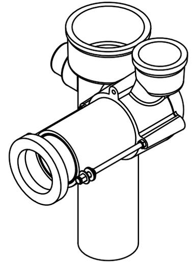
FOR 2" NO-HUB AUX. INLET, EITHER CUT IN FIELD OR SPECIFY (-50) THREADED (-54)
