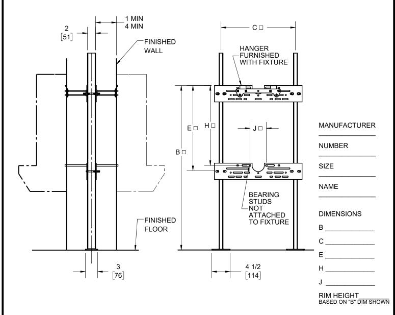
RECOMMEND ALL FEET BE SECURED TO FLOOR WITH 1/2" BOLTS AND ANCHORS BY OTHERS.
