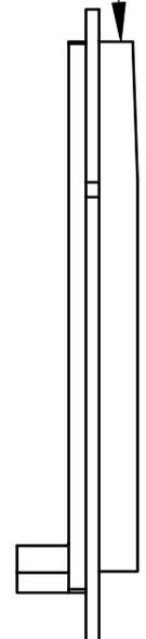
INSERT FLAT HEAD SCREWS THRU THESE SLOTS AND INTO BOSSES ON MALE END OF CHANNEL
