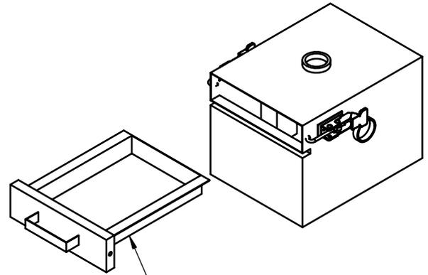
DRAWER TYPE SOLIDS BASKET WITH  $\varnothing 5/32$  [4] HOLES SIDES AND BOTTOM
