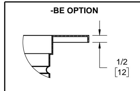
OUTLET O.D. DESIGNED TO FIT CLOSELY WITH I.D. OF NO-HUB CAST IRON PIPE
