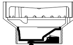
E Series Round Tractor Strainer shown with Optional (-J) Backwater Valve Formerly EJ Series Strainer
