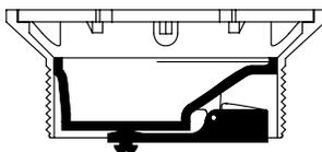
A Series Round Strainer shown with Optional (-J) Backwater Valve Formerly AJ Series Strainer
