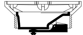
S Series Square Strainer shown with Optional (-J) Backwater Valve Formerly SJ Series Strainer
