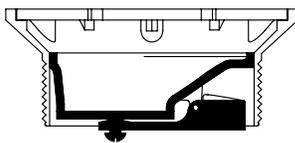
A Series Round Strainer shown with Optional (-J) Backwater Valve Formerly AJ Series Strainer
